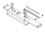
Using supplied key wrench to adjust armature plate to approx. 3 mm of gap between magnet surface.
