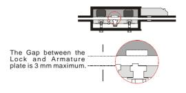
Using supplied key wrench to adjust armature plate to approx. 3 mm of gap between magnet surface.
