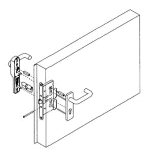
Cross bar with square spindle to drive a mortice lock.
