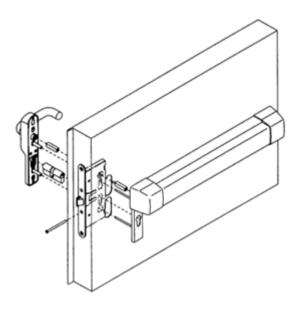
Handle with square spindle to drive a mortice lock.
