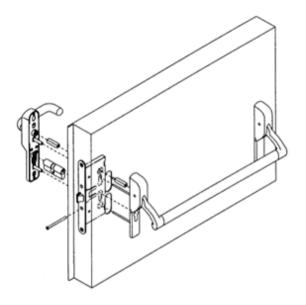
Push bar with square spindle to drive a mortice lock.
