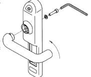
Select the cylinder plate that matches the lock c/c distance (72 or 92) and insert it in its seat. If half cylinders or no cylinder is used, insert the blind plate.
