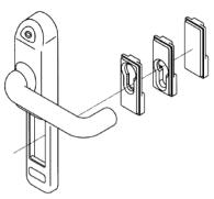
Fix the rear plate with the screws, being sure to position the fitting bushes in positions compatible with the lock.
