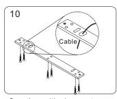
Once the position is correct, use the screws to permanently mount the mounting plate, And drill the cable access hole.
