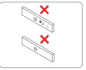
Damage to the mating surfaces may reduce the efficiency of the lock and cause rust.
