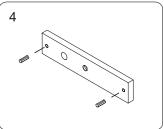
Insert the guide pins into the armature plate. The guide pins will prevent the armature plate to pivot around.
