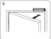
Close the door. Measure the correct position by bringing the armature plate close to the contact surface of the electromagnetic lock.
