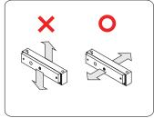
During the installation procedure, it is important to make sure that the working direction of the armature plate has to be facing toward the contact surface of the electromagnetic lock in order to have the maximum holding force.
