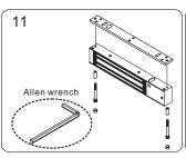
Use the Allen wrench to screw the Fixing screws and Brass Sleeves through the bottom of the electromagnet into the mounting
