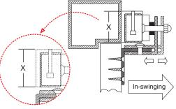
The "X" value is 48mm which is the minimum requirement width of the door frame for Model No.13700 600 lbs electromagnet locks.
