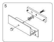
Put one rubber washer between armature plate and the Z part of LZ bracket, and place them over the 8mm armature screw.
