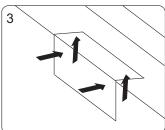
Place the template against the door and frame. Drill two holes in the frame on the template.
