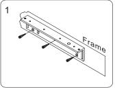
Find a mounting location on the door frame for the L bracket. Make sure that the door is still closable.
