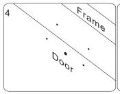
Drill two holes in the frame and three holes in the door as indicated on the template.
