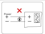
Do not install a diode in parallel with any magnetic lock. A diode will cause a delay when releasing the door and residual magnet to occur.
