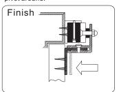
Once the position is correct, use the screws to permanently mount the Z part of LZ bracket on the door. This should be the last step.
