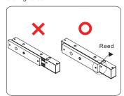
The contact surface of the electromagnetic lock and the armature plate has to be completely attached; otherwise, the reed, which located in side the electromagnetic lock, will not be detected. It will result an incorrect output message for the bond sensor.
