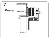
Turn on the power of EM-Lock, and let the armature plate bond to the EM-lock. Adjust the position between the Z bracket and the door frame.
