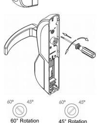
• Using the key, it is possible to mechanically enable the electric handle.
