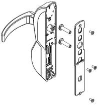
If one of the fixing bushes is placed to the cylinder height, tighten the supplied nylons gauge in the back part of the bush (see figure).
