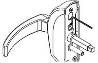
Tighten the screws previosuly reduced to complete the installation. Make sure the striking parts are free to move and do not hit parts of the door or obstruct the bar mechanism.
