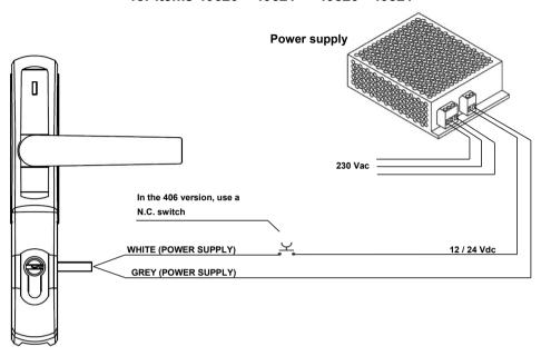
"AC" power supply with direct electricity activation for items 40620 – 40621\* – 40820 - 40821\*
