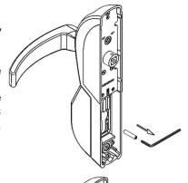
Fix the back plate with the appropriate screws and make sure the fixing bushes are in the correct position in front of the fixing holes on the bar.
