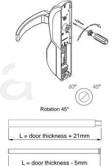
Fix the back plate with the appropriate screws. Check if the fixing sockets are in the correct position, compatible with the fixing holes on the panic bar
